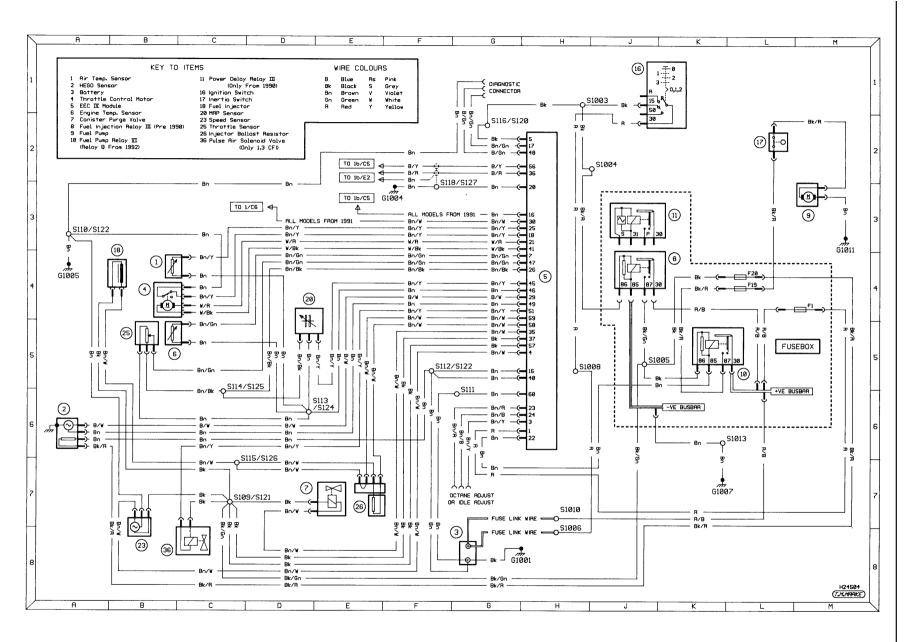
Diagram 1c: Typical 1.1/1.3/1.4 CFi fuel injection
